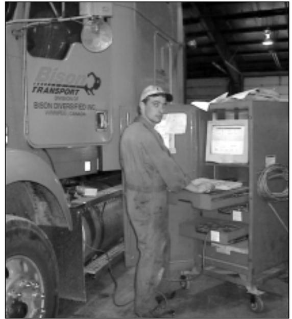
***A Bison Transport mechanic uses a computer to optimize the running performance of a truck, critical to its plan in reducing emissions. Employee "buy in" to the plan is also important, and company management has not found this difficult to achieve.***
