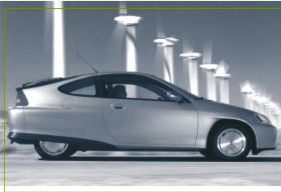
The 2001 Honda Insight, the first gasoline-electric hybrid vehicle sold in North America, has substantially reduced emissions and has an average fuel economy of 64 mpg.
