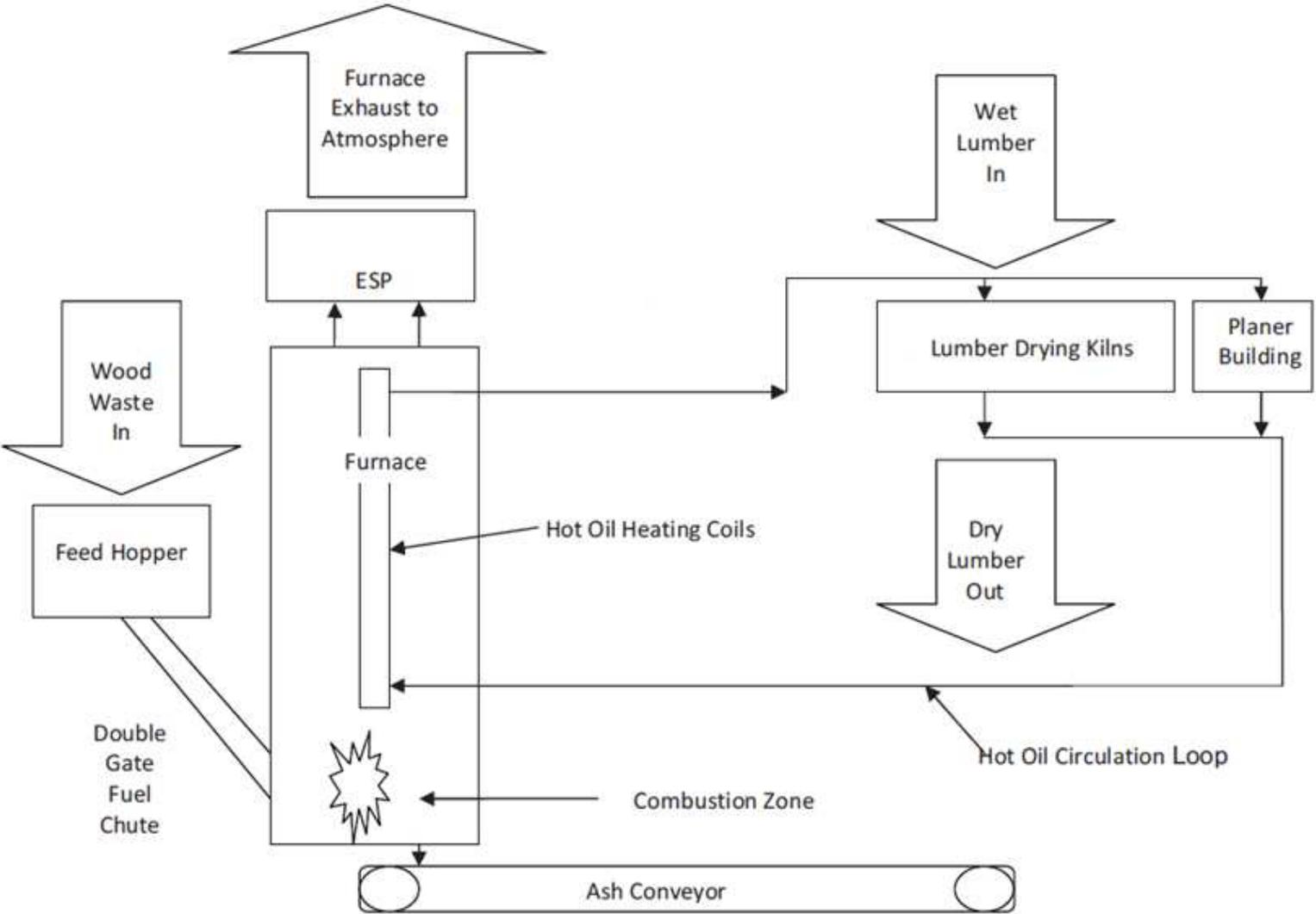
Figure-2: Simplified flow diagram of THF in Edson Forest Products
