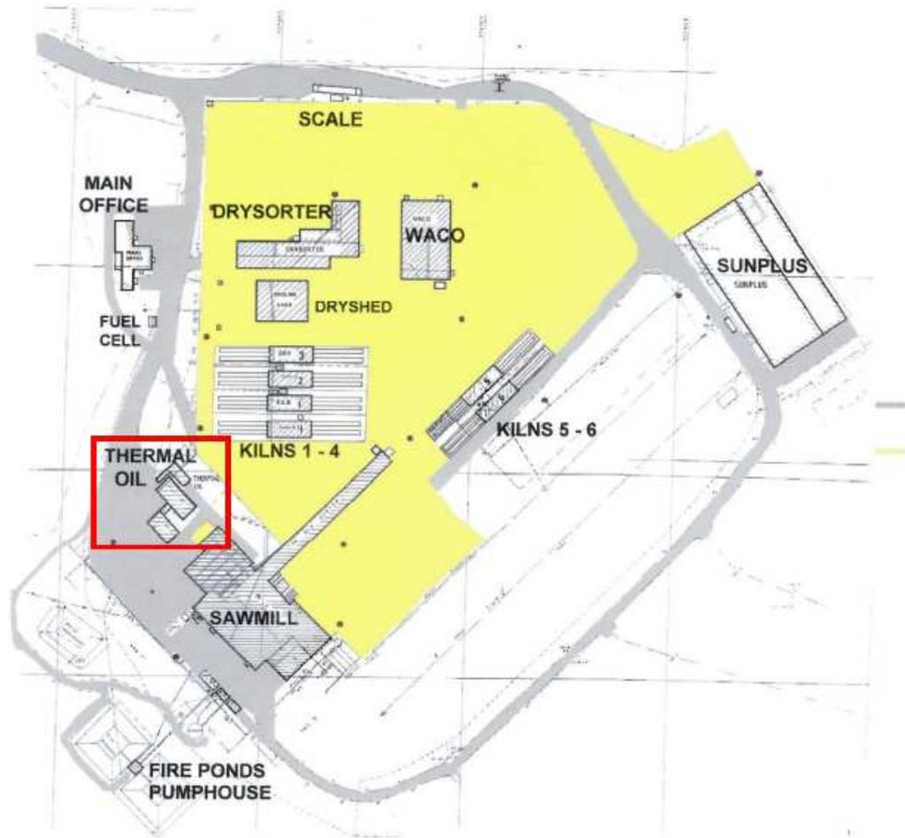
Figure-1: Project boundary of Thermally Heated Fluid furnace at Edson Forest Products
