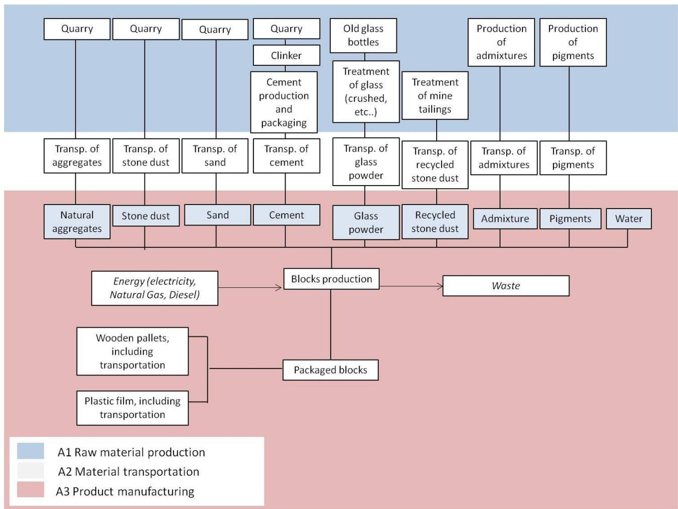
**Figure 1: System boundaries for Standard and Noble® blocks - Cradle-to-Gate LCA**
