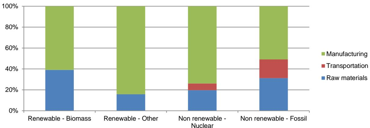
**Figure 3: Contribution of life cycle stages to the environmental impacts of 1m<sup>3</sup> of Standard blocks, Energy consumption**
