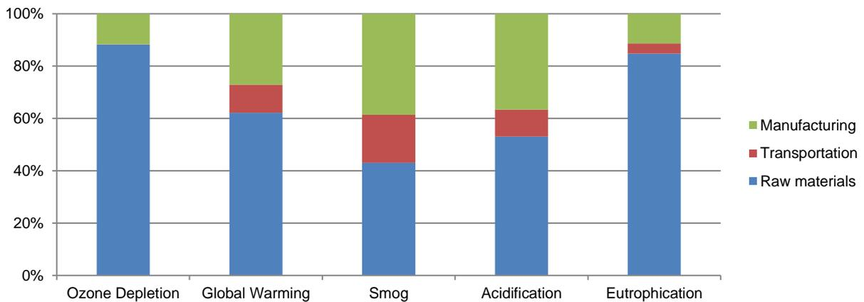
**Figure 2: Contribution of life cycle stages to the environmental impacts of 1m<sup>3</sup> of Standard blocks, TRACI indicators**
